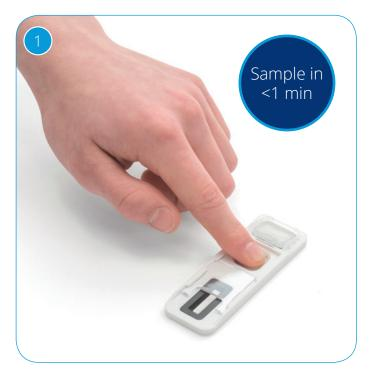
The fingerprint sample is collected by firmly pressing all ten fingertips in sequence onto the Intelligent Fingerprinting Cartridge sample pad for five seconds each.
