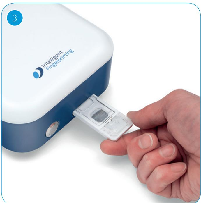
The Cartridge is placed in the Intelligent Fingerprinting DSR-Plus for analysis.
